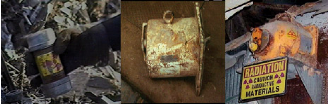
Figure 2 Examples of radioactive sources from demolition sites
