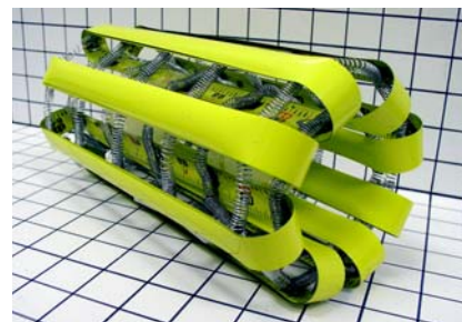
The Whole Skin Locomotion device is inspired by the mobility motion of an amoeba. Credit: Dennis Hong
