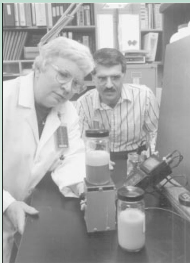
Sharon Haynes, Union Carbide senior laboratory technician in South Charleston, and Albert Joseph, development scientist, inspect an emulsion after Union Carbide's new TRITON SP series surfactant has been deactivated, separating the emulsion into two distinct materials. When used in laundry detergents, the deactivation allows for rapid separation of major pollutants that can be recycled or treated, and the clean effluent discharged.
