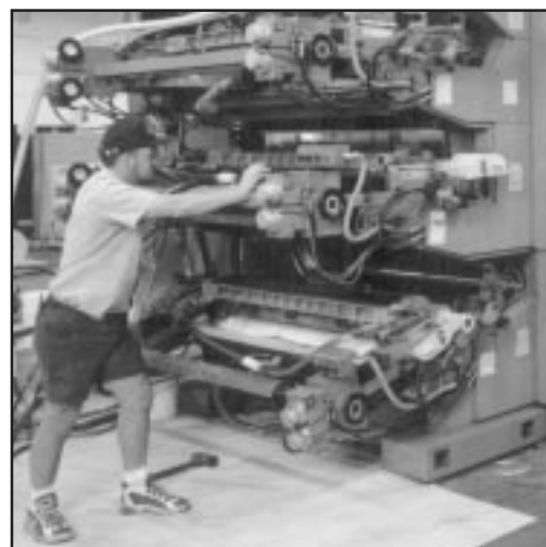
A press worker attends a central impression flexographic press during a DfE Flexography Project on-site performance demonstration.
