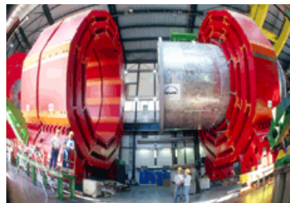
The Central Yoke of the CMS Detector. Credit: CERN
