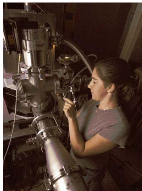
A graduate student prepares the beta-Nuclear Magnetic Resonance apparatus for an experiment with rare isotopes. While the general methods employed in beta-NMR are the same as used today in medical applications of Magnetic Resonance Imaging, experiments with rare isotopes are up to 14 orders of magnitude more sensitive by detecting the emitted beta particle, when the rare isotope decays. Credit: NSCL at Michigan State University
