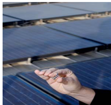
A sample of an organic solar cell fabricated on a flexible plastic substrate. An array of conventional silicon solar cells is shown in the background. Credit: Nicole Cappello, Georgia Tech.
