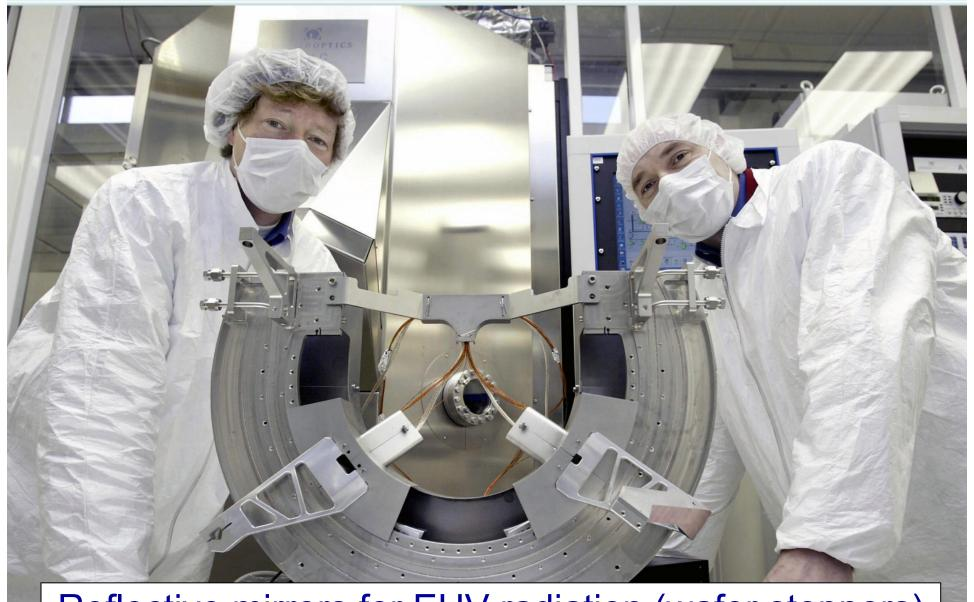
Reflective mirrors for EUV radiation (wafer steppers)
