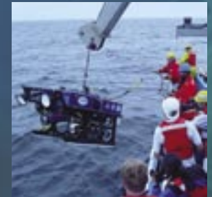
A ROV is lowered over the side of the R/V Connecticut during a survey of the wreck of the steamship Portland . Photo: Anne Smrcina/SBNMS
