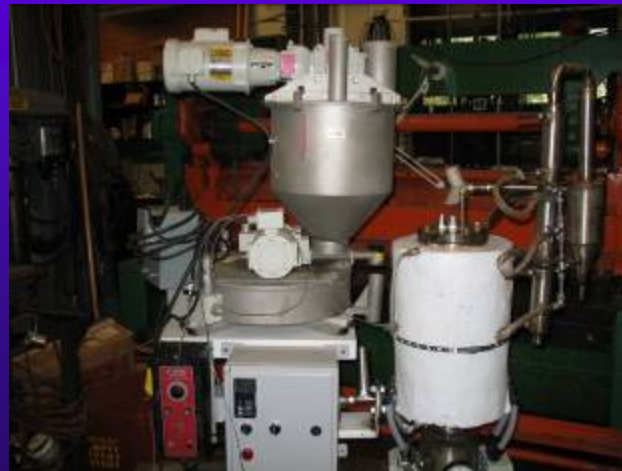
ERRC's 3" Fluidized Bed Pilot Pyrolysis Unit
