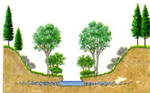
Streambanks and channel in good condition
