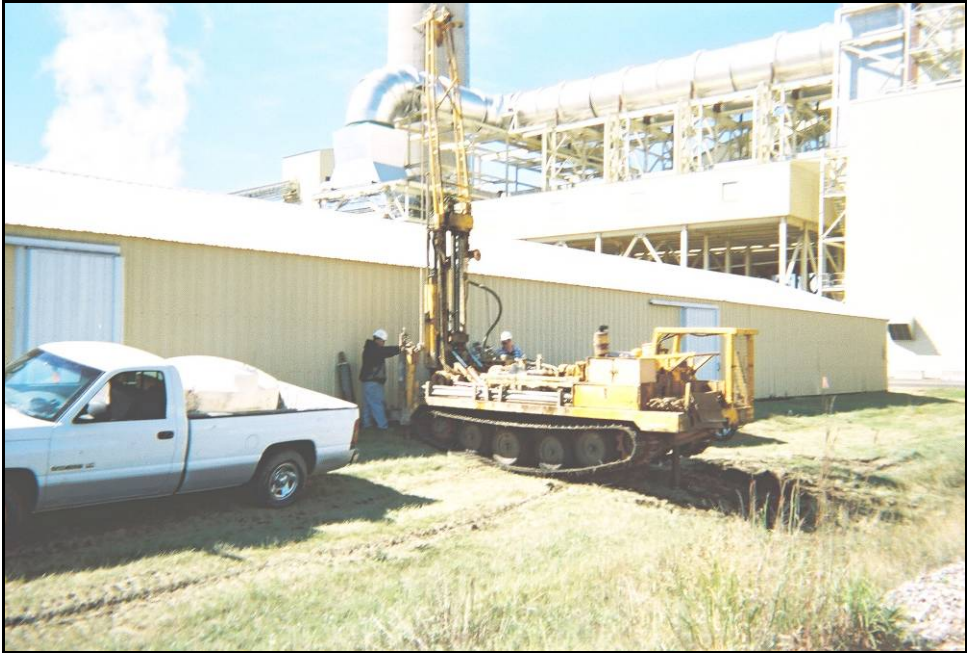
Figure 3-10. Typical Coring Tracked Vehicle.
