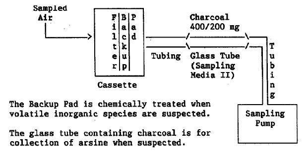
If arsine is suspected, use a minimum amount of tubing to connect the cassette to the arsine sampling tube.
