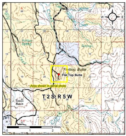
Flat Top Butte Community Pit is located east of Highway 95, 4 miles east of the Oregon border; T 2 S , R 5 W,Section 21, W 1/2, NW 1/4, SW 1/4; E 1/2, SW 1/4, NW 1/4. It is located within Miocene Rhyolite of the Silver City Range, which is reddish-brown and flow layered. The rock at this location is good for decorative stone. The area of disturbance is approximately 18.4 acres, and the permit is for 40 acres.
