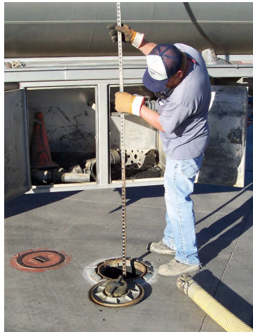
Measuring the product level in a tank
