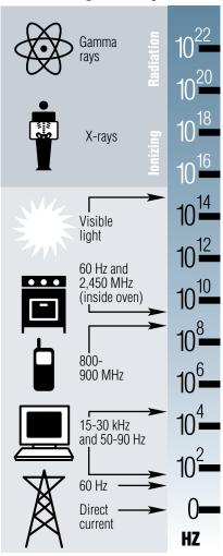
Frequency is shown in Hertz (Hz). 1 Hz = 1 cycle per second. (Note that  $10^4$  means 10x10x10x10=10,000 Hz, etc.) kHz = kilohertz = 1000 Hz, MHz = megahertz = million Hz.
