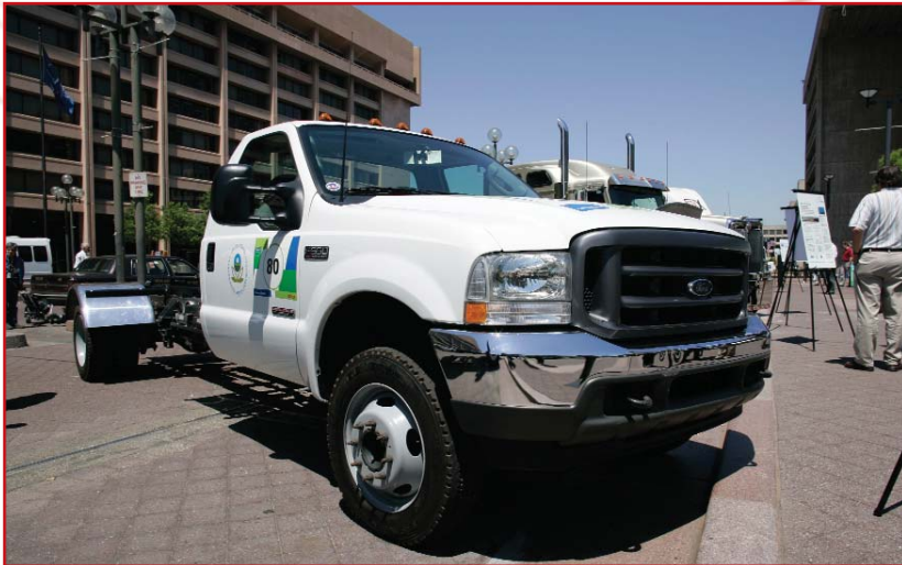
EPA's Mild Hydraulic Hybrid Truck in a Medium Duty Delivery Truck Chassis
