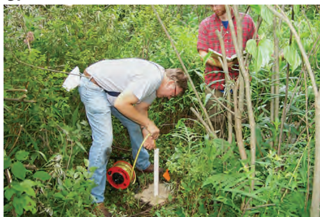
Figure 45. Silver Brook Café water source in Sandisfield, Massachusetts, showing A , collection structure at upper center and seepage melting snow at lower right, westward view (photograph by Bruce Bouck, Massachusetts Department of Environmental Protection); B , blue pump intake in collection structure; and C , measuring water level in small-diameter observation well.
