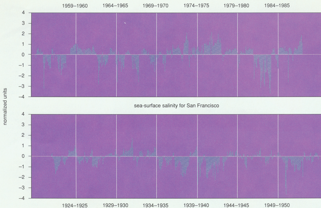
Figure 3. Understanding of estuarine dynamics in San Francisco Bay is taxed by the salinity fluctuations, which occur at several different time scales. Shown here are the salinity anomalies at Fort Point, near the mouth of the bay. The long-term salinity trend has been removed from the data, leaving only the monthly fluctuation in salinity.
