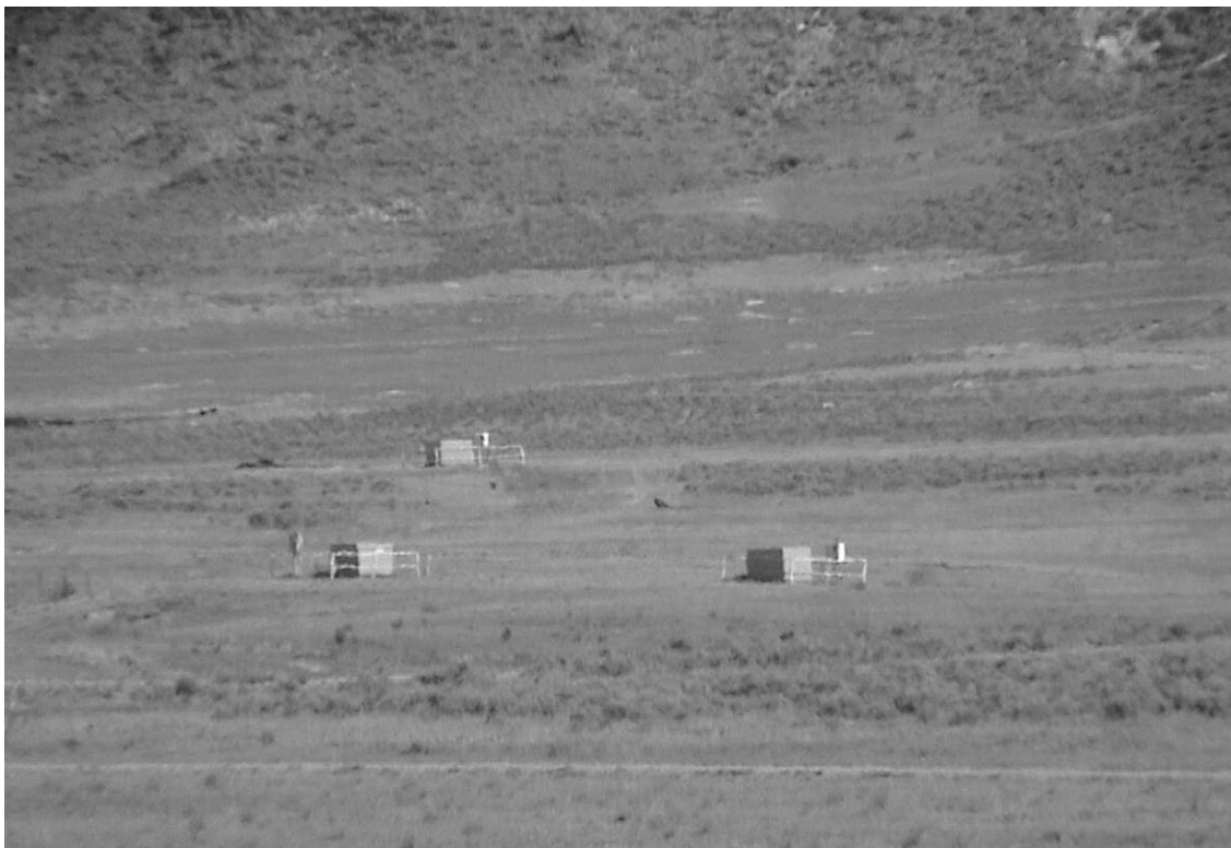
Three CBNG well heads forming a field pod near Decker, Montana. Each well is drilled to a different depth and into a different layer of coal.
