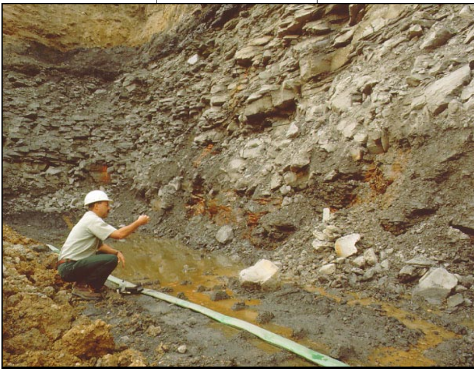
Office of Surface Mining inspector at work in Tennessee testing acidity of water in the mine pit.
