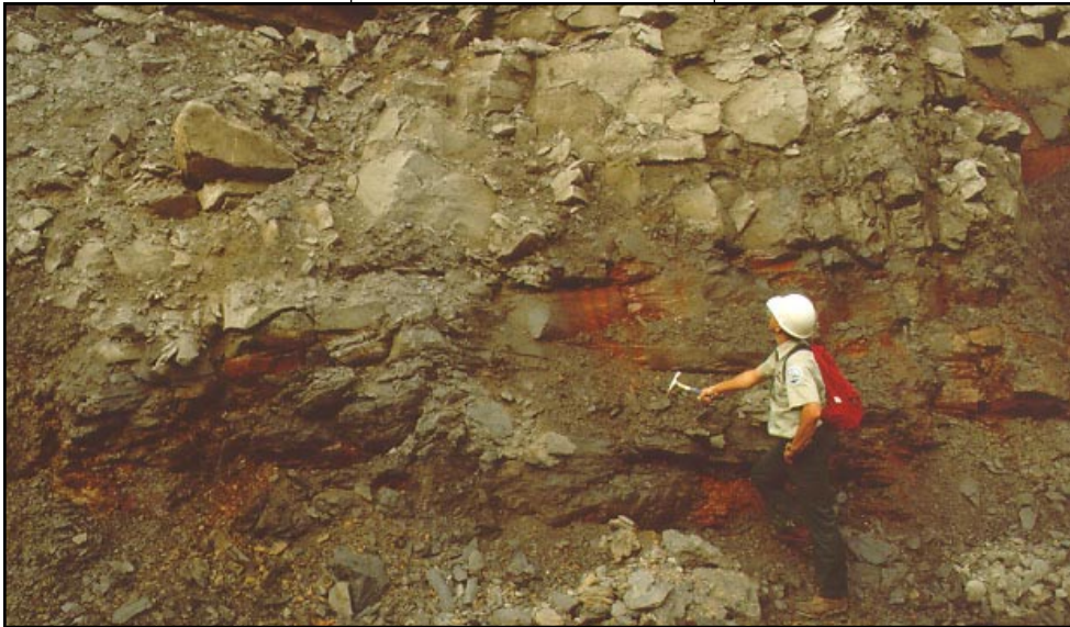
Mine inspector examines acid seeps in the highwall.
