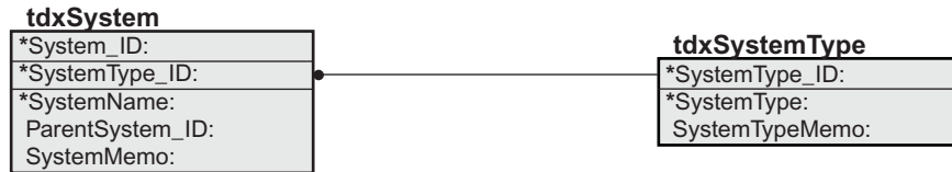
Figure 19. System subject area tables, fields, and relationships. (Box represents a field coming from another table, an asterisk represents a required field, and a black ball indicates a foreign key. See figure 18 for explanation of box color.)
