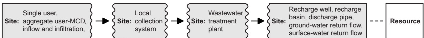
Figure 11. Network 6: Diagram for modeling collection and return by a simple community-wastewater system with single users, aggregates of users, and inflow and infiltration. (Dotted line represents a Site-Resource association, solid line represents a conveyance, and an arrowhead shows the direction of water movement.)
