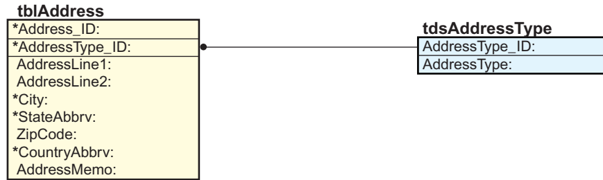
Figure 21. Address subject area tables, fields, and relationships. (Box represents a field coming from another table, an asterisk represents a required field in data tables, and a black ball indicates a foreign key. See figure 18 for explanation of box color.)
