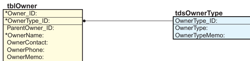
Figure 20. Owner subject area tables, fields, and relationships. (Box represents a field coming from another table, an asterisk represents a required field in data tables, and a black ball indicates a foreign key. See figure 18 for explanation of box color.)
