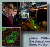
Researchers at Michigan State University have developed ultrashort pulse lasers and the technology used to improve biomedical imaging. The cells inside a mouse kidney are displayed here using 15 femtosecond
