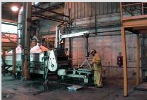
Fig. 4. Enclosed and exhaust ventilated star caster
