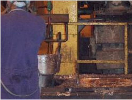
Lifting recently cast lead blocks from mold
