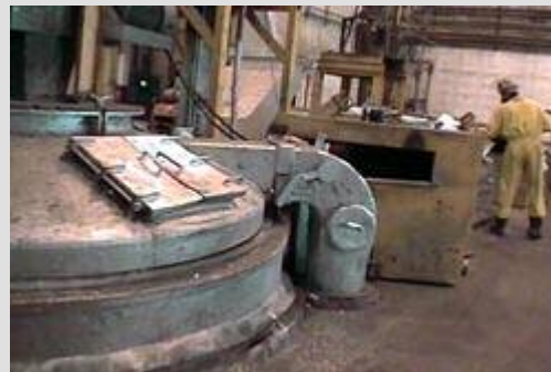
Fig. 1. Manual removal of dross may expose workers to lead dust and fume
