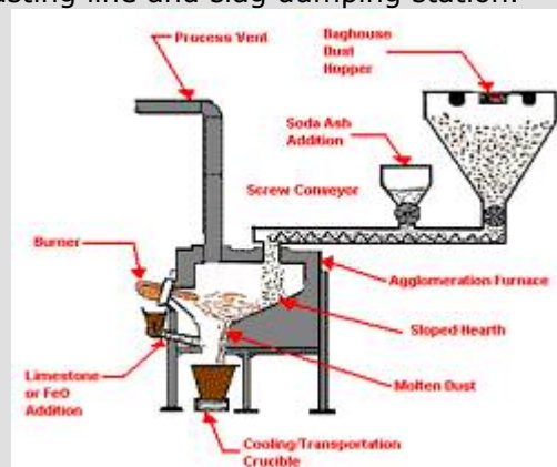
Click for larger view of agglomeration furnace
