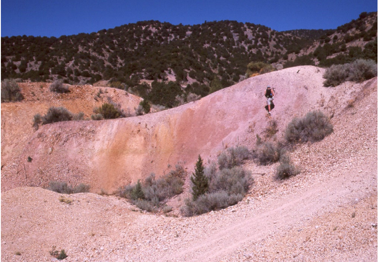
Figure 41 (this page, top). Open-pit clay mine in Clay Canyon, southern Oquirrh Mountains. Large envelopes of highly argillized rock containing goethite and kaolinite (pictured here) surround small zones of alunite. Location: 40^{\circ}16'52.85''\text{N} , 112^{\circ}10'43.24''\text{W} .
