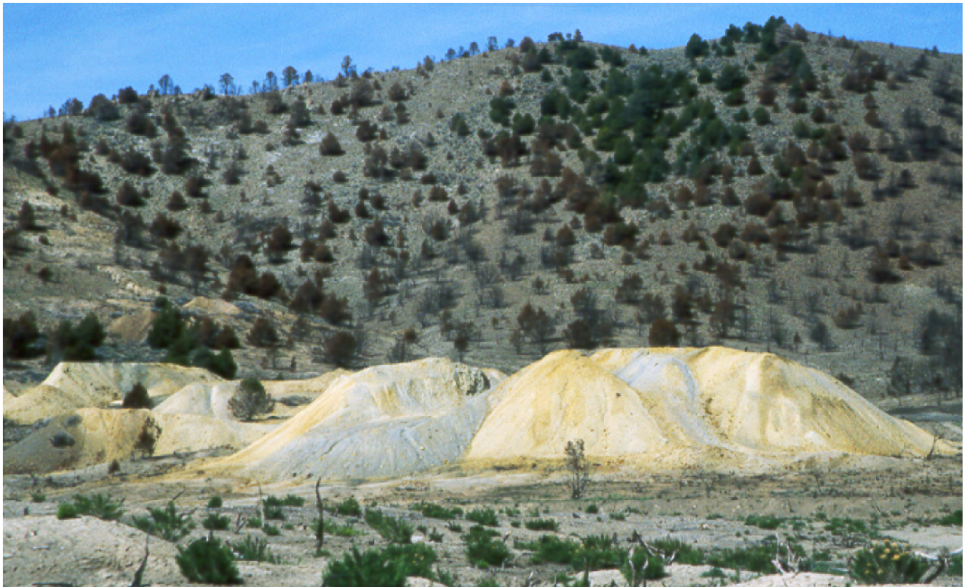
Figure 20. Waste-rock piles with yellowish and yellow-green coatings of jarosite at the Swansea mine site (location shown in figs. 13–16 ) near Silver City. These piles, which reach >6\ \text{m} in height, are typical of mine waste in the Tintic mining district. Piñon and juniper trees and bushes that burned during the 1999 range fire are visible in the background on hills underlain by the Swansea Quartz Monzonite and Silver City Monzonite.
