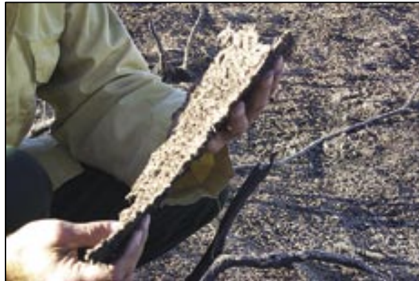
Figure 2.2. Hydromulch is applied to form a smooth dense mat on the soil surface (USDA/USFS, 2006).
