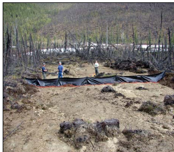
Figure 2.6. A silt fence, designed to monitor soil movement, installed across a recent burn and landslide (Guyer, 2006).
