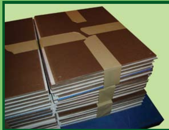
Photographs of rice hull / plastic composite sign substrate example shown: 6.5mm thickness.
