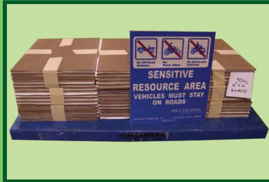
Photographs of rice hull / plastic composite sign substrate example shown: 6.5mm thickness.
