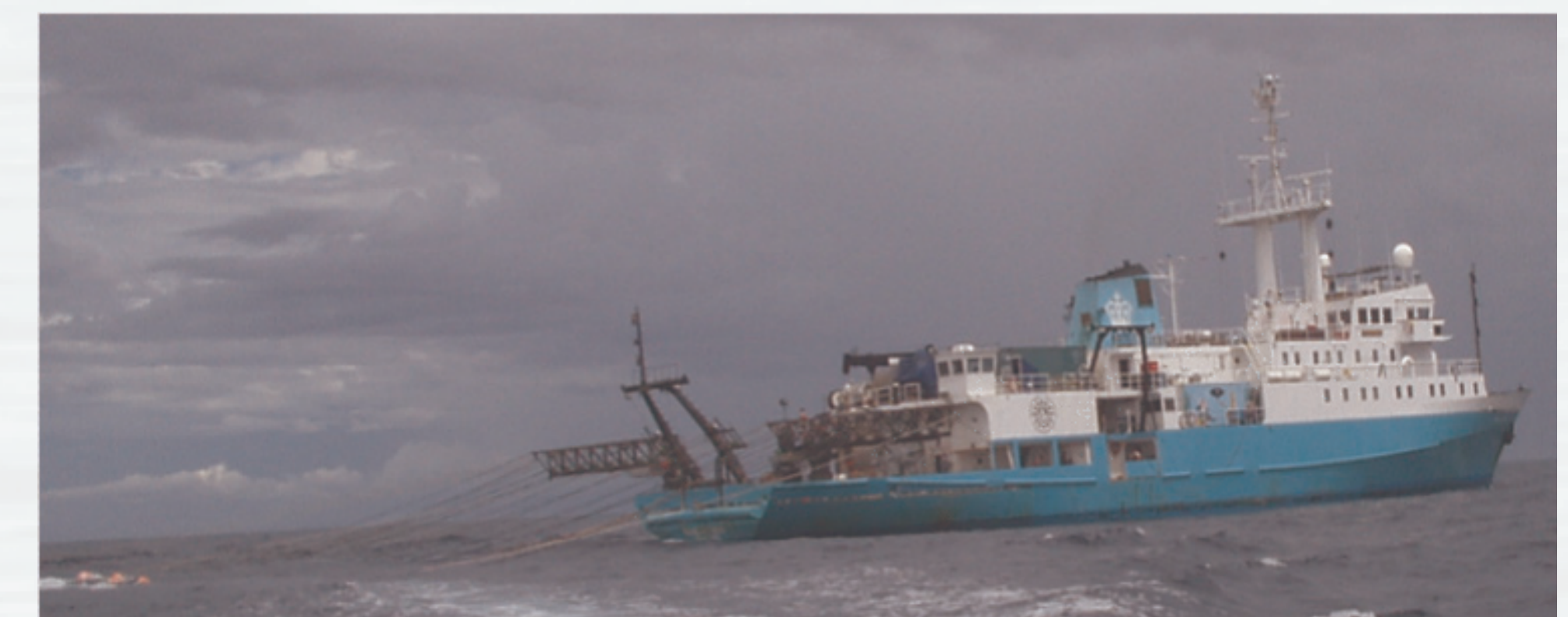
The R/V Maurice Ewing towing an airgun array during a 2004 marine seismic study. The airgun lines are towed from the two black transverse booms seen in this photo.
