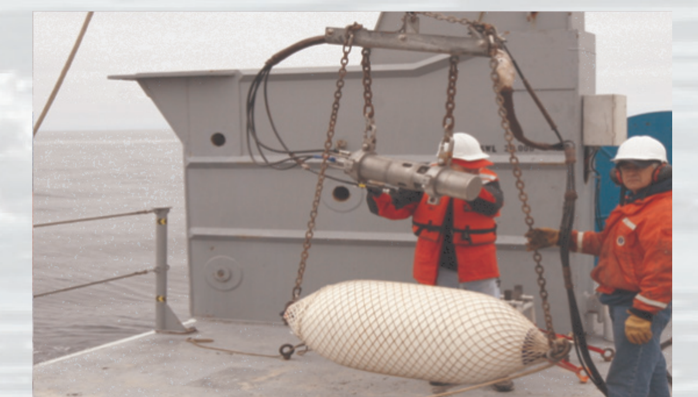
An engineer prepares to deploy a single airgun from the vessel as part of an “array” of airguns. Each airgun is suspended about 8 m below the water surface from a white or pink float shown here. The energy to the airguns is compressed air supplied by compressors on board the source vessel.
