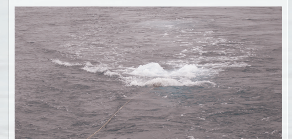
A close-up of the seismic airgun releasing air bubbles at the water surface immediately after a pulse of air is released.
