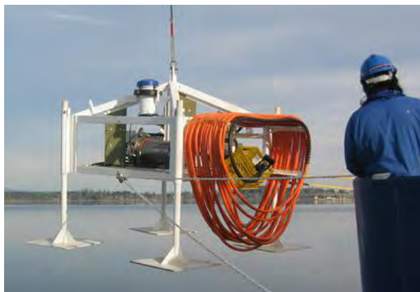
Figure 2-11 Representative Junction Box (Jbox)
