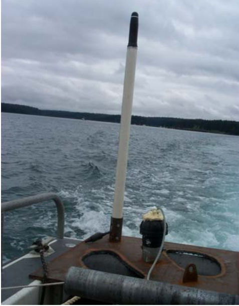
Original hydrophone installation
