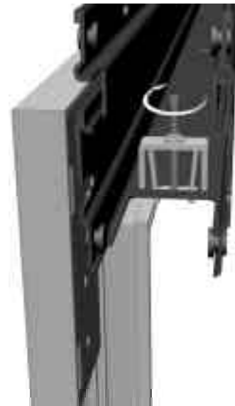
TURN DISLODGE- MENT INSERT SCREW TO EXPAND PRONGS
