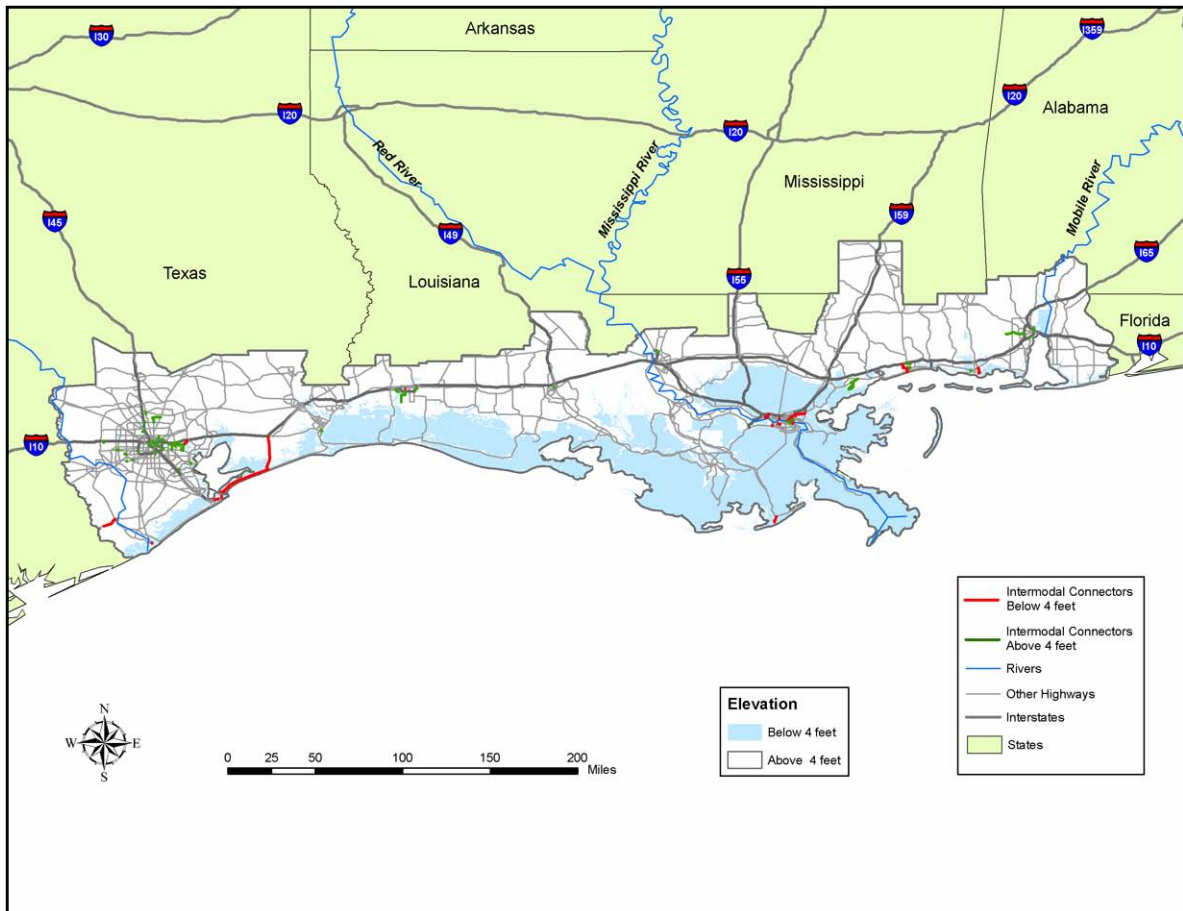
Figure 4.3 NHS Intermodal Connectors at risk from a relative sea level rise of 122 cm (four feet). (Source: Cambridge Systematics analysis of U.S. DOT data)
