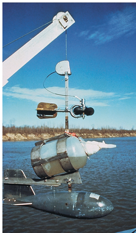
A noncontaminating isokinetic sampler (made entirely of Teflon®) was used to collect samples of bed sediment, water, and suspended sediment.
