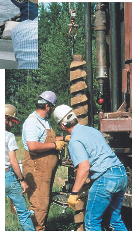
Drilling for soil samples near Bemidji, Minnesota
