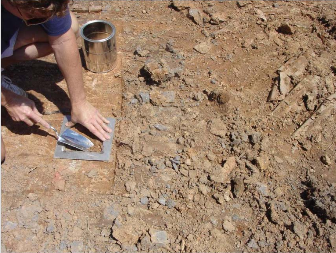
Figure 5-1. Soil sampling after the NESHAP demolition.
