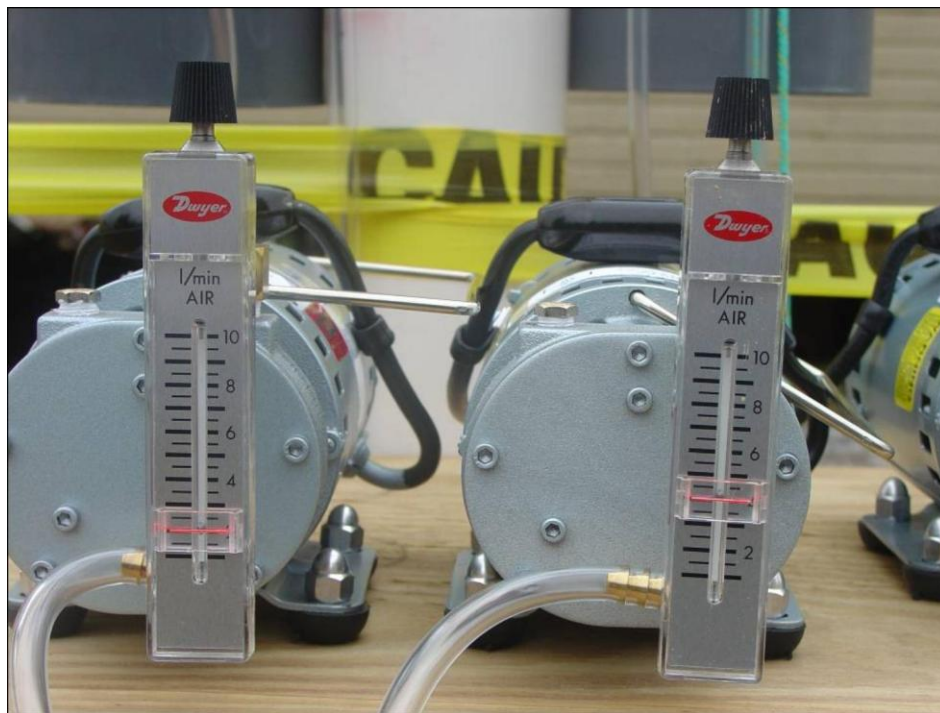
Figure 4-15. Pre-calibrated rotameters with sight gauges set at two and four liter/min.
