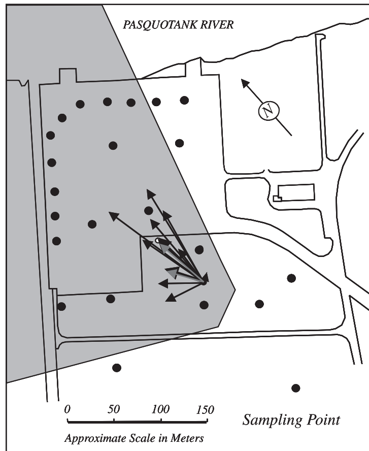
Figure 3.1. Variation in the direction and magnitude of ground water flow at an MTBE site in Elizabeth City, North Carolina. The arrows represent the distance that water would move in one year, based on the direction and hydraulic gradient present in a particular round of sampling. Some of the arrows are shaded grey to allow them to be distinguished from the other arrows. The origin of the arrows is the center of the LNAPL source area. The black dots are locations of monitoring wells. The shaded area includes all the monitoring wells with concentrations of MTBE above 20 \mu\text{g/l} .
