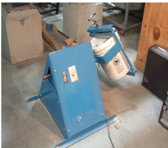
Figure 5. Mixing Fly Ash Prior to Obtaining Aliquots for Laboratory Analyses.
