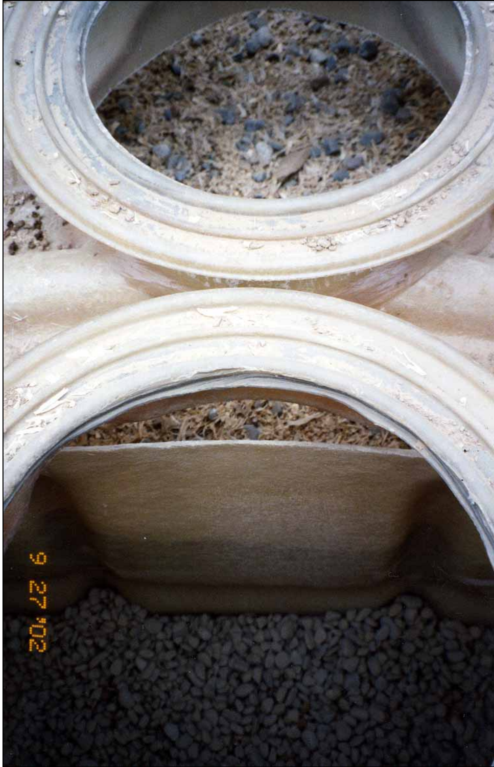
Figure 2-16. Whole bone apatite/gravel media before submerging it with water. Note vertical baffle/partition visible in photo.
