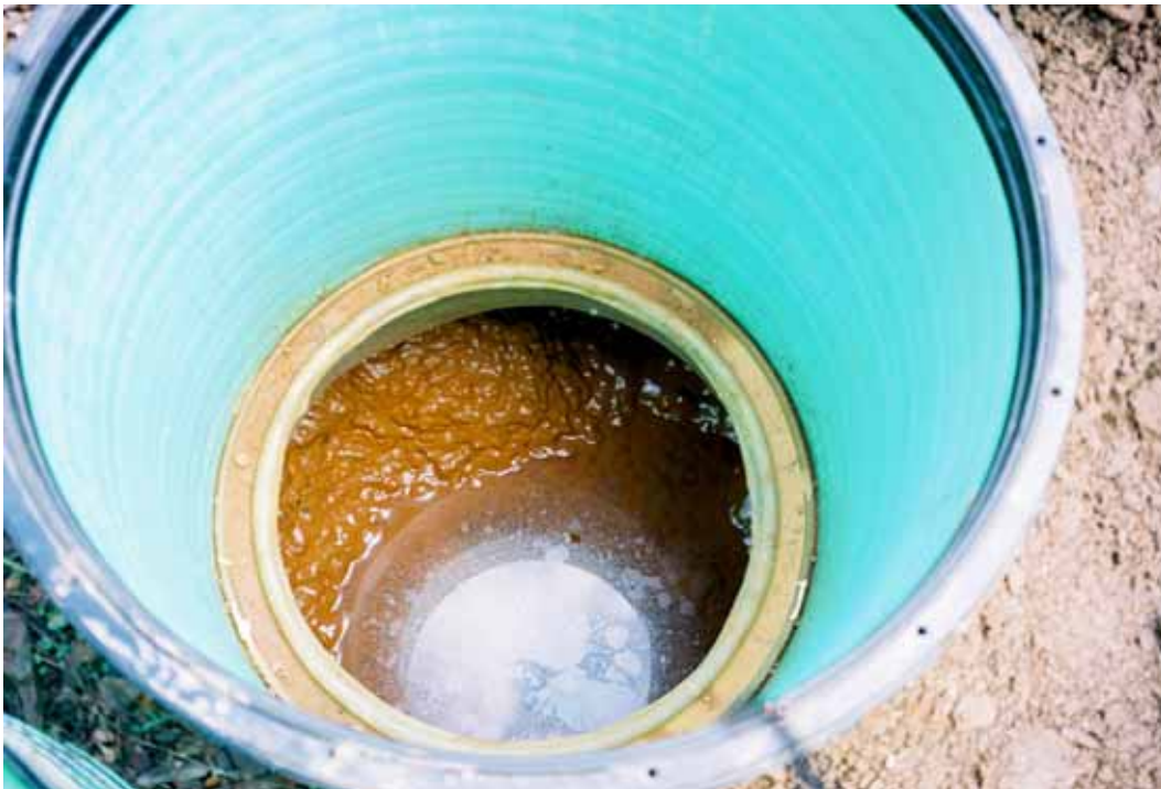
Figure 5-4. Tank 4 (center cell) just prior to the solid phase (total digest) sampling showing the ferrihydrite coated surface.
