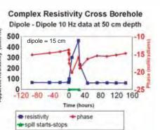
Anomalies were observed with multiple geophysical methods indicating changes occurred in different physical properties of the formations with the presence of the PCE. A monitoring approach utilizing multiple, different geophysical methods and scientific expertise could provide unique detection and identification of subsurface PCE.
