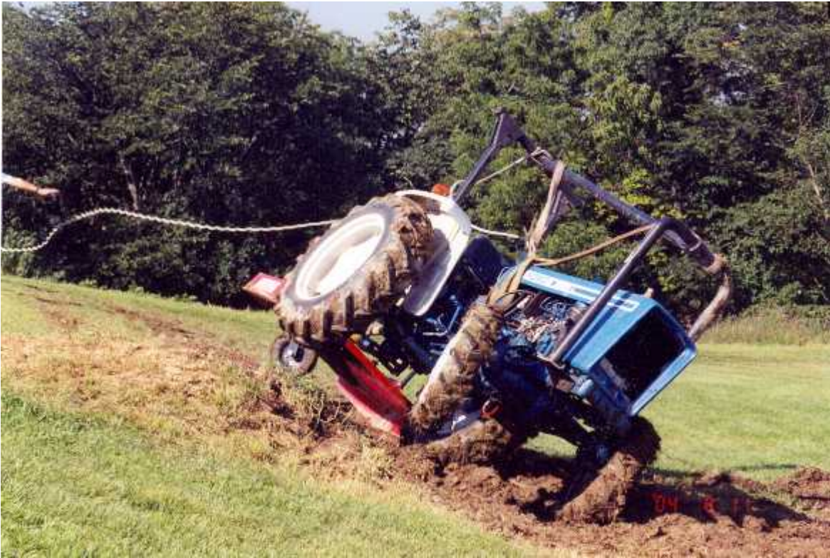
Figure 1 - Side Overturn Test with Rear Deck Mower During Statistical Testing
