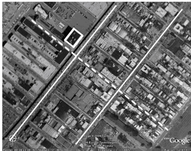
Fig. 1 Aerial photograph of the neighborhood in Brooklyn, NY, studied in the B-TRAPPED field study. The 12-story tower is indicated with a white rectangle. Solid white lines mark two major avenues, corresponding to Avenue 2 (left) and Avenue 3 (right) in the wind tunnel and CFD models. The dashed white line highlights one of the streets parallel to the wind direction.
