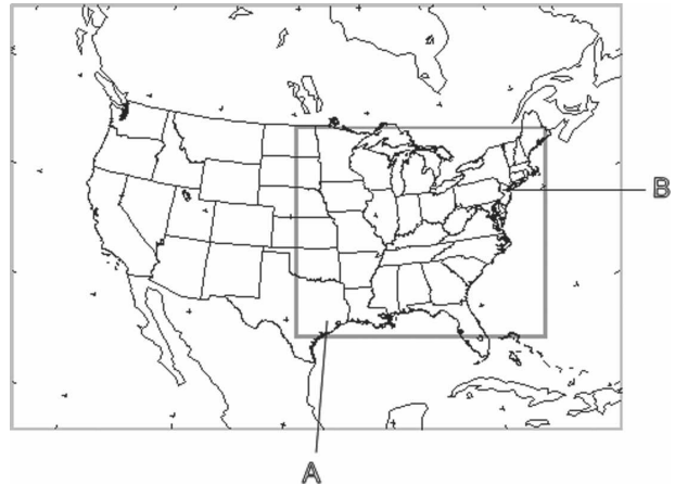
FIG. 1. Modeling domain encompassing the continental (36-km grid spacing) and eastern (12-km grid spacing) United States. Results from grid cells marked “A” and “B” are presented in Figs. 3 and 5, respectively.
