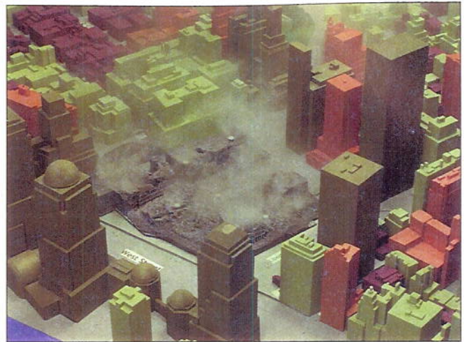
Figure 2. Model of Manhattan used in wind tunnel simulations of pollutants emitted from the site of the collapsed World Trade Center towers.
