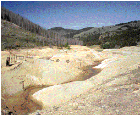
Tailings filling the High Ore Creek valley, Boulder River watershed southwestern Montana in 1997. The creek eroded a channel through the tailings, washing them down to the Boulder River and enriching the water with metals.
