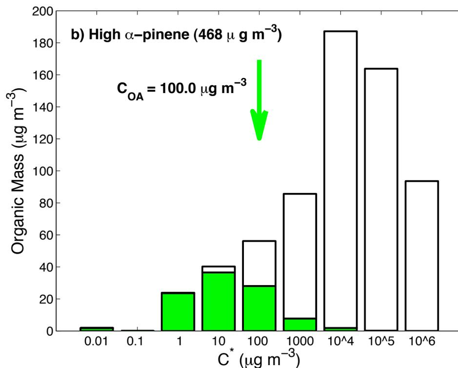
Partitioning changes with mass loading:  $\times 18$  total loading =  $\times 100 C_{\text{OA}}$ .
