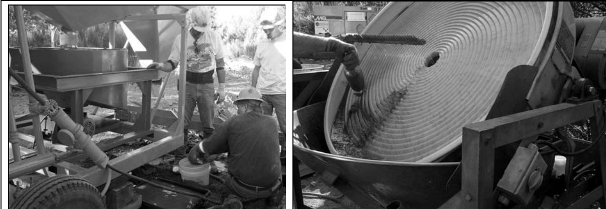
Some equipment used in separating heavy mineral sands and mercury contaminants. The spiral wheel in the far right photo is used in the final separation of mercury from less dense mineral sands. The recovered mercury is deposited in a pan below, where it is then collected and shipped to an authorized mercury recycler.
