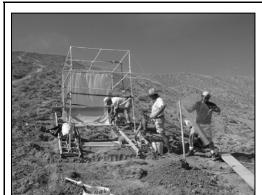
Soil scientist and crew set up a rainfall runoff simulation test to assess impacts of OHV activity on saline soils in the Gunnison Gorge, Colorado.
