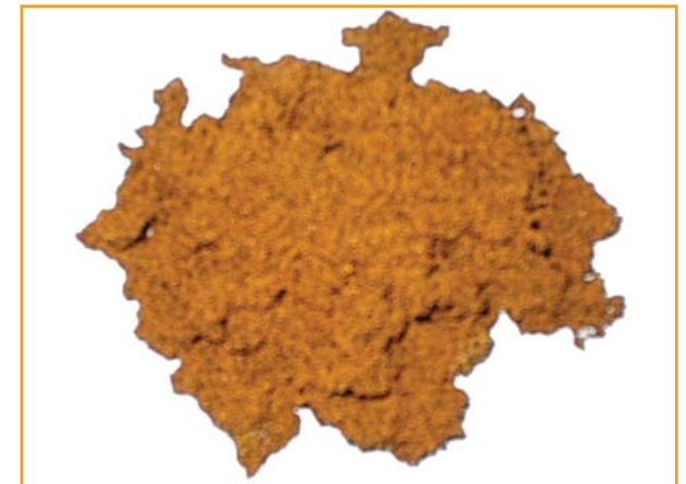
HIX, developed by VEEtech, P.C., is a family of polymeric-inorganic hybrid sorbents that can selectively capture all forms of arsenic and other co-contaminants from drinking water.
