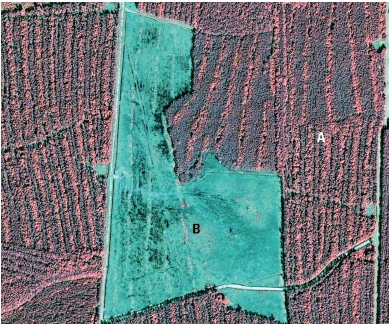
Figure 20. Trees planted in rows with uniform crown height (A) and block clear cuts [blue-green feature in center (B)] were indicators of managed forest plantations. Color infrared Ikonos satellite image, Virginia 2004. Courtesy of Space Imaging Corp.
