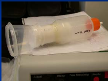
Filtering large volumes of tap/source water spiked with MS2 bacteriophages
