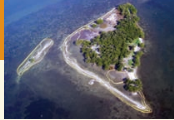
Pelican Island is ringed with a yellow turbidity barrier that reduces sedimentation in surrounding water and protects adjacent sea grasses while helicopters drop bucks of shells in the area. (Mike Marshall/Coastal Resources Group)
