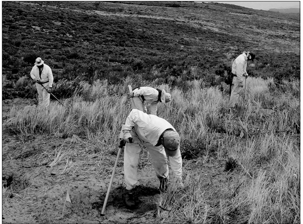
Figure 2: Workers Searching for UXO at the Former Fort Ord Using Hand-Held Detection Devices
